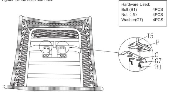
Step 10 – Turn over the seat frame and insert it to base(E).
