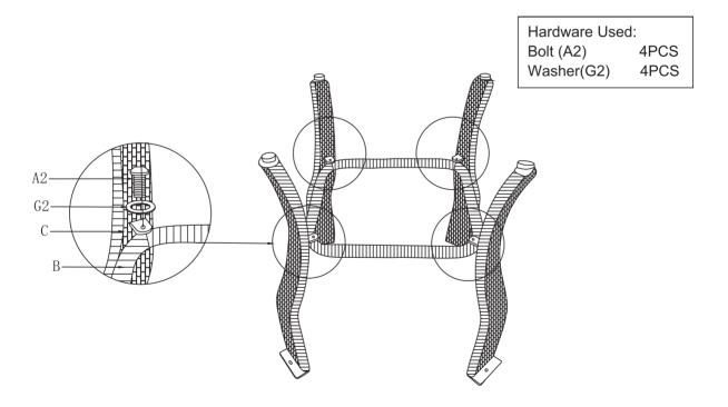
Step 2 – Assemble table rim (A) to table leg (C) by using bolt (A2) and washer (G2). Repeat this step for the other table leg (C).
